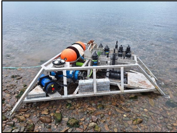
Figure 6: FAST-2 platform equipped with five Innovasea acoustic receiver technologies (with duplicates for redundancy), an ADCP and hydrophone for recording flow speed and underwater noise.
